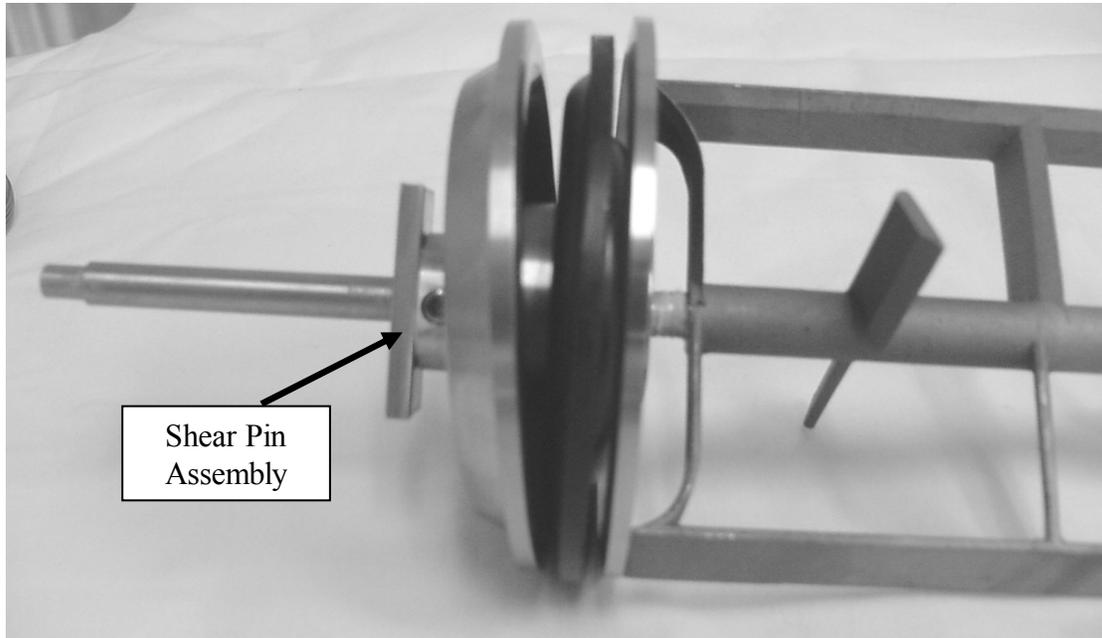
5. Install the complete paddle assembly into the slurry cup.
